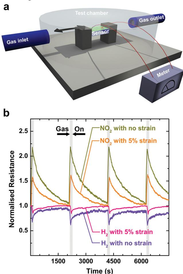
**Figure 3.** Testing of the ZnO gas sensors: a) Schematic representation of a sample during test in a chamber with controlled gas flow and in situ resistance measurement. b) Room temperature response of the microtactonic sensor to hydrogen and nitrogen dioxide in relaxed and stretched states (gray/shaded areas represent gas exposure for 80 s).
