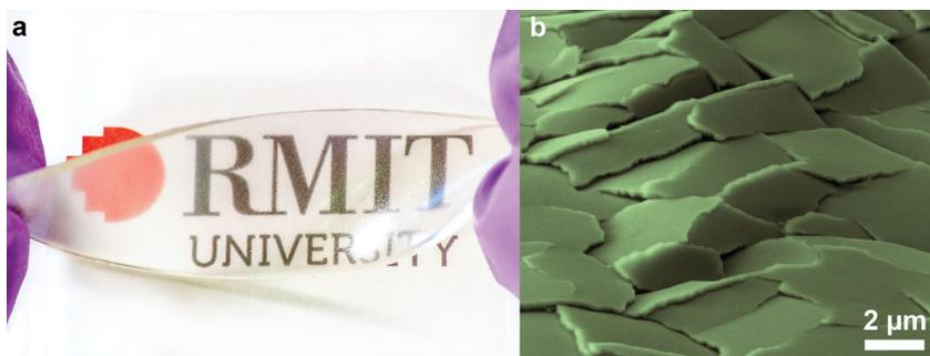
**Figure 2.** a) Transparency and the ability to flex and twist a microtactonic ZnO device is shown in this photograph. b) False-color scanning electron image of the surface-cracked microtactonic surface of ZnO.
