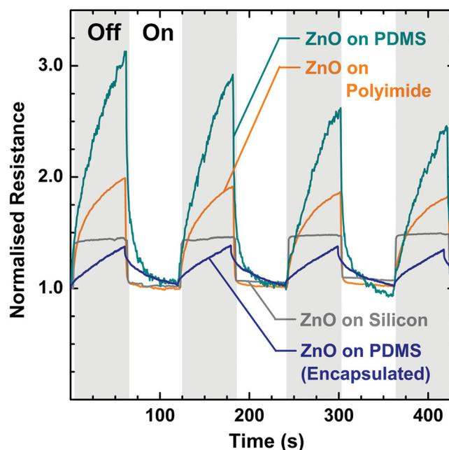
**Figure 5.** Sensitivity comparison of surface engineered ZnO-UV sensors. UV sensitivity of ZnO sensors fabricated on silicon, polyimide, and transferred to PDMS with identical synthesis parameters.
