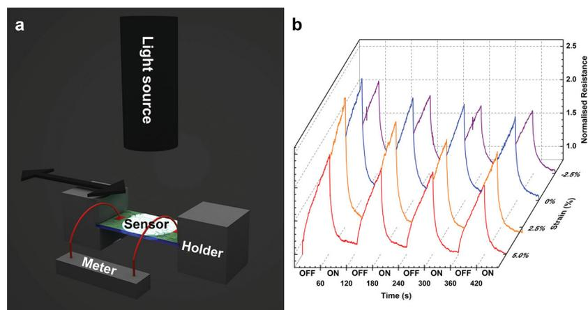
**Figure 4.** Optical sensing response of microtectonic ZnO to ultraviolet radiation. a) Schematic of testing arrangement with high energy UV illumination and microscale stretching capability for in situ measurements. b) Normalized resistance under cyclic exposure to darkness (OFF state) and broadband UV illumination of 1 sun (ON state) for different levels of uniaxial strain.
