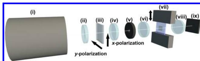
**Figure 2.** Schematic of arrangement for optical characterization of dielectric resonator metasurfaces. Components include (i) white light source; (ii) collimating lens; (iii) sheet polarizer; (iv) 40 $\times$  objective; (v) 50  $\mu\text{m}$  pinhole; (vi) 20 $\times$  objective; (vii) tunable dielectric resonator array sample on a stretching stage; (viii) collimating lens; and (ix) fiber-coupled spectrometer.
