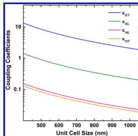
Figure 7. Influence of metasurface geometry on coupling coefficients. The coupling coefficients (in logarithmic scale) as a function of the square unit cell size (side length).
