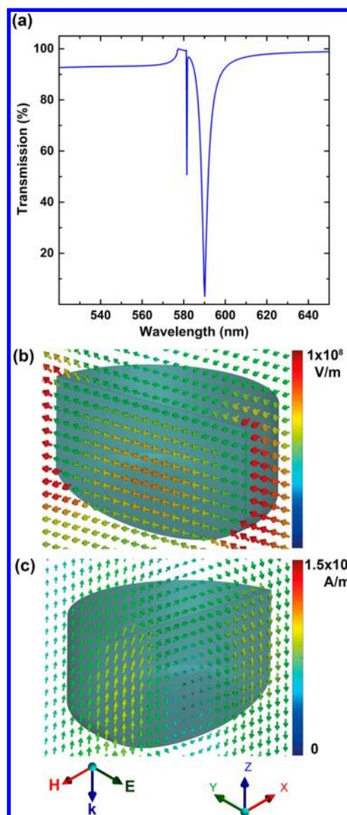
**Figure 3.** Resonant electric dipole response of a dielectric resonator in unstrained PDMS matrix. (a) Simulated transmission of the unstrained array sample, for a normally incident wave with  $E$ -field along the  $y$ -direction. Simulated (b)  $E$ -field on the  $y$ - $z$  plane and (c)  $H$ -field on the  $x$ - $z$  plane of the resonators in an infinite unstrained array corresponding to the resonance peak in (a).
