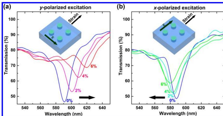
Figure 5. Polarization-dependent transmission spectra of the metasurfaces with increasing applied strain. (a)  $y$ -Polarization excitation transverse to applied strain. (b)  $x$ -Polarization excitation parallel to applied strain.
